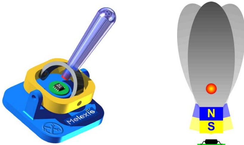
Figure 3 - Typical application of MLX90333
