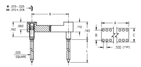
**Description:** DIP Socket Wrapost Tail 1 Level Wrapost Tail Open Frame Accepts .015-.025" Leads Plating Code: Shell Plating: 10 μ" Gold over 100 μ" Nickel Inner Contact Plating: 30 μ" Gold over 50 μ" Nickel Packaging:
