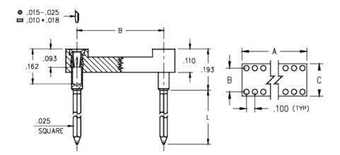
**Description:** DIP Socket Wrapost Tail 2 Level Wrapost Tail Open Frame Accepts .015-.025" Leads Plating Code: Shell Plating: 10 μ" Gold over 100 μ" Nickel Inner Contact Plating:
