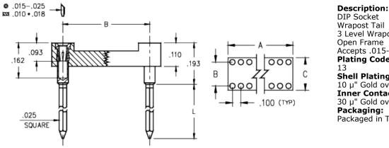
3 Level Wrapost Tail Accepts .015-.025" Leads Plating Code: Shell Plating: 10 µ" Gold over 100 µ" Nickel Inner Contact Plating: 30 µ" Gold over 50 µ" Nickel Packaged in Tubes
