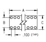
Description: DIP Header Interconnect Open Frame Through Hole Plating Code: 10
