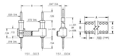
**Description:** DIP Header Interconnect Open Frame Through Hole Plating Code:
