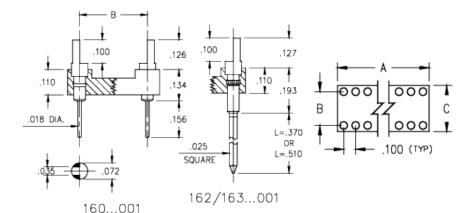
**Description:** DIP Header Slotted Header Solder Tail Open Frame Through Hole Plating Code: 90 Shell Plating: 200 μ" Tin/Lead(93/7) over 100 μ" Nickel
