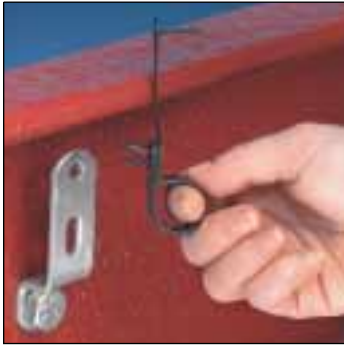
1. Install into 1/8" (3.2mm) thick panel or bracket with a hole diameter of 0.281" (7.1mm) typical clearance hole for 1/4" (6mm) bolts.
