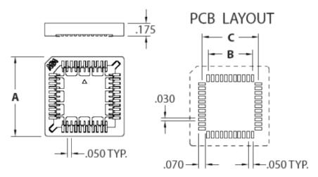
FOR PRINTED CIRCUIT DRILLING PATTERNS
