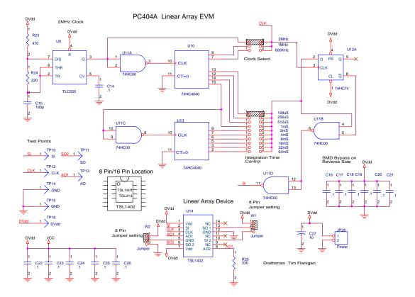
Figure 1 - PC404A Schematic Diagram
