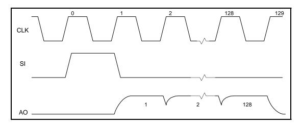
Figure 2 - System Timing (AO output for TSL1401 shown)
