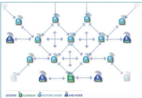
IP-Link 3000& 3200 dongles support Star, Cluster-Tree and Mesh Topologies
