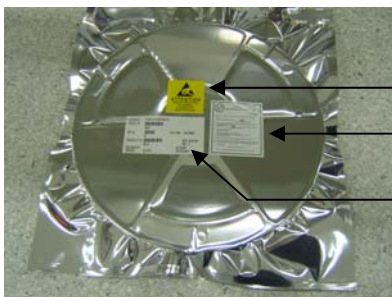
Moisture Barrier Bag With Labels
