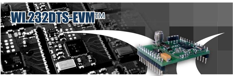
Evaluation Wireless Module 915 MHz, 152.34 kbit/sec.
