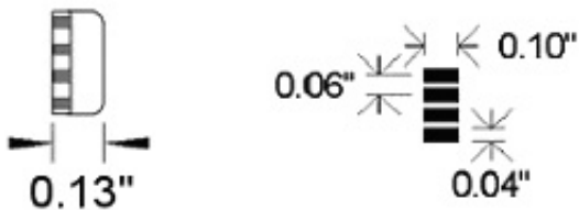
Figure 3: Suggested Pad Layout
