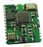
allows quick PC connectivity to a Wi.232DTS™ network. The Wi.USB-DTS™ is USB-powered and provides the same highly configurable, highperformance wireless link as our other Wi.232DTS™-based products. The Wi.USB-DTS™ is perfect for: Wi.232DTS™ based sensor networks requiring PC/ Laptop Interface, point-to-point longe-range PC/Laptop communications, AMR basestation/mobile unit is Wi.232DTS™ base meter network.
