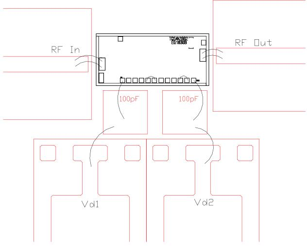
This configuration is for a self-bias logic pad current search with connections for bin #1. See Table IV for alternate bin # to get the current of typical  $80 \pm 10\%$  mA.
