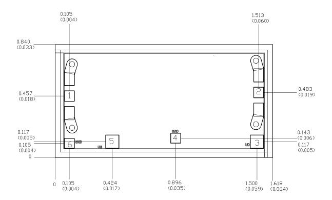
Units: Millimeters (inches) Thickness: 0.050 (0.002) (reference only) Chip edge to bond pad dimensions are shown to center of bond pad Chip size tolerance: +/- 0.051 (0.002) RF Ground is backside of MMIC
