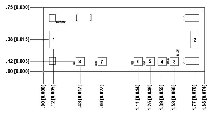
Units: millimeters [inches] Thickness: 0.10 [0.004] (reference only) Chip edge to bond pad dimensions are shown to center of bond pads. Chip size tolerance: ±0.05 [0.002] RF ground through backside
