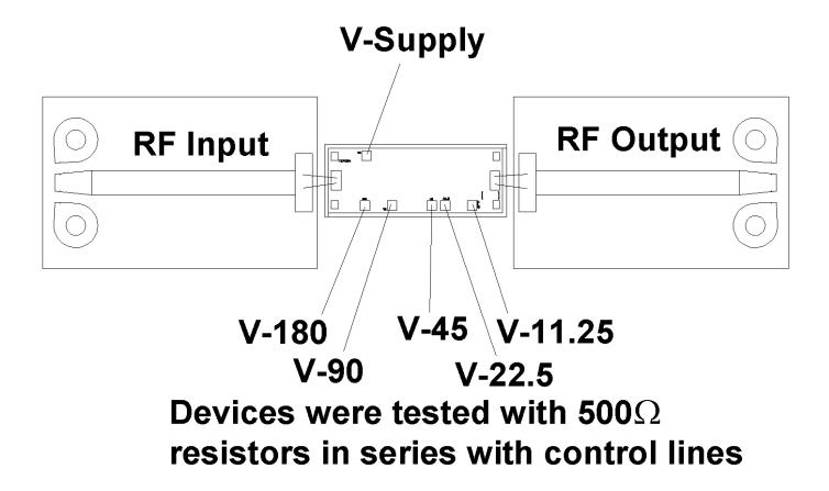
GaAs MMIC devices are susceptible to damage from Electrostatic Discharge. Proper precautions should be observed during handling, assembly and test.
