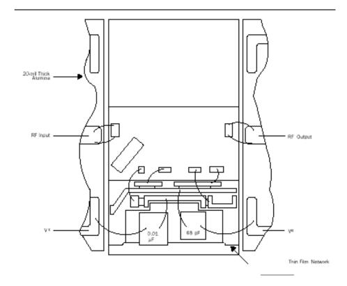
RF connections: Bond two 1-mil diameter, 25-mil-length gold bond wires at both RF Input and RF Output for optimum RF performance.
