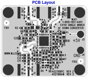
Circuit Board Material: .014" FR-4, 4 layers, .062" total thickness
