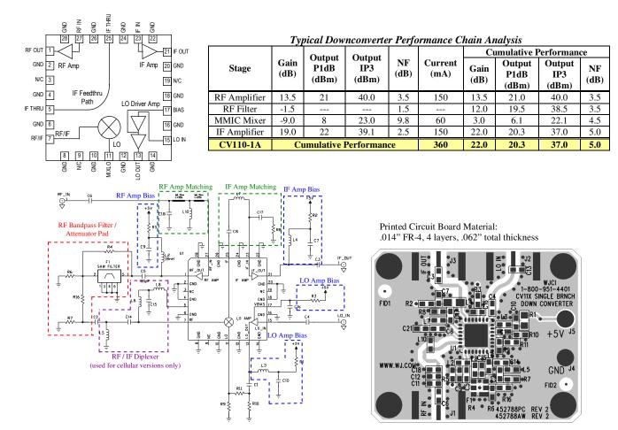
**CV110-1A**: The application circuit can be broken up into four main functions as denoted in the colored dotted areas above: RF/IF diplexing (purple), amplifier matching (green), filtering (red), and dc biasing (blue). There are various placeholders for chip components in the circuit schematic so that a common PCB can be used for all WJ single-branch converters. Additional placeholders for other optional functions such as filtering are also included.
