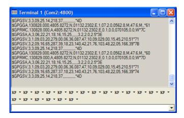
Figure 5: GPS Cockpit NMEA terminal with NMEA data
