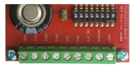
Figure 8: Terminal block (picture turned by 90°)
