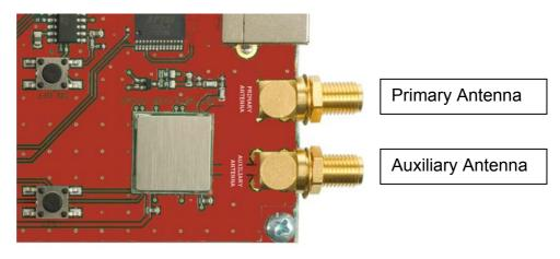
Figure 6: Primary and Auxiliary Antenna Connector
