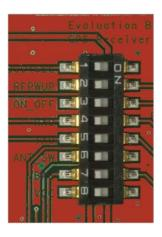
Figure 9: DIP switches
