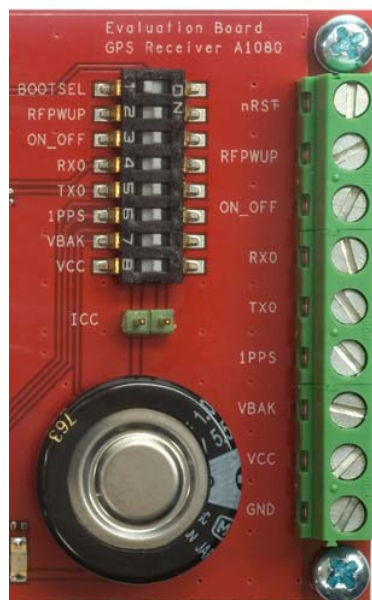
Figure 8: Screw connectors J3,J4,J5
