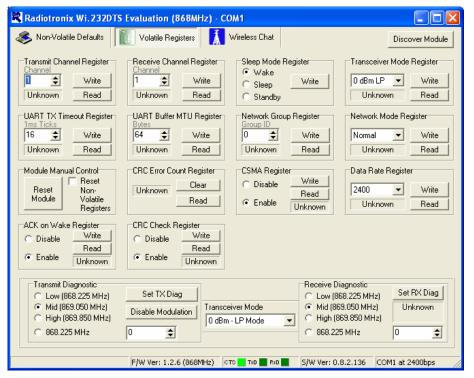
In this page, you can change the Volatile settings of the module. Values programmed into these registers are lost of power-down.
