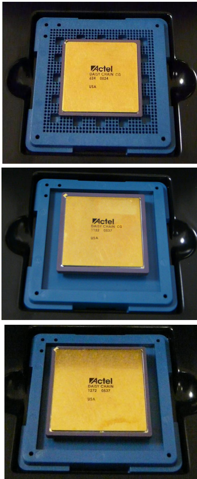
Figure 10 • From Top to Bottom: CG624, CG1152, and CG1272 in their Respective Tray Carriers
