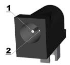
At the PWR pin should be applied voltage 4.5VAC or +(6-9)VDC.
