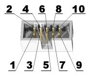
**PDI** Input **Programming Data In.** This pin is used for data input while programming the MCU through ICSP.
