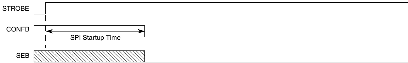
Figure 22. Valid Sequence from Standby/LVD Mode to Configuration Mode
