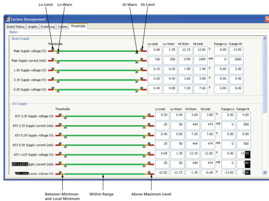
Figure 4-2. Setting Thresholds by Slide Marker
