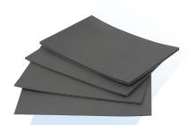
Q-ZORB PN 2240, RFSW-S-060-FR-PSA is a flexible elastomeric magnetic absorbing material. The material is designed to perform well for surface current attenuation. It can be used to lower the Q of cavities and reduce EMI. It is easily bonded using contact adhesives or it can be supplied with a pressure sensitive acrylic adhesive (PSA).
