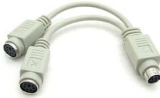
Figure 4-26 Y-Cable use for both Keyboard and Mouse
