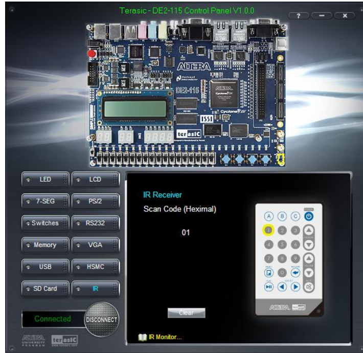
Figure 3-14 Testing the IR receiver using remote controller
