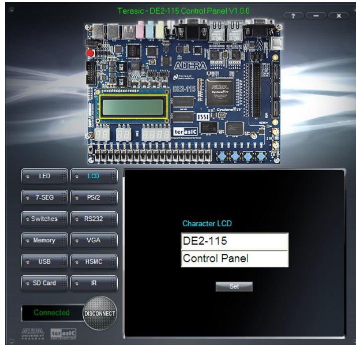
Figure 3-5 Controlling the LCD display
