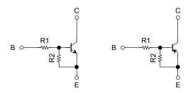
R1:  $10 \text{ k}\Omega$ R2:  $10 \text{ k}\Omega$
