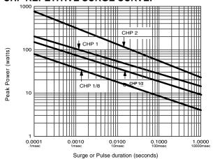
Note: Use for repetitive pulses where the average power dissipation is not to exceed the component rating at 70°C. Surge handling capacity for lowrepetitive surges may be significantly greater than shown above. Contact factory for recommendations.
