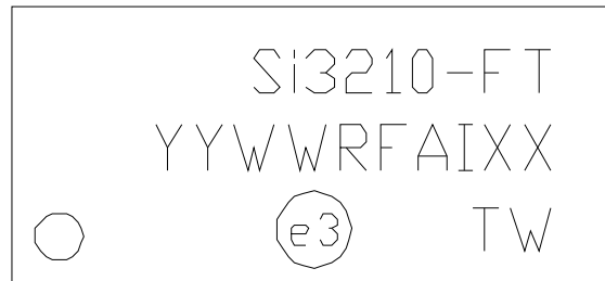
Figure 40. TSSOP Top Mark Diagram
