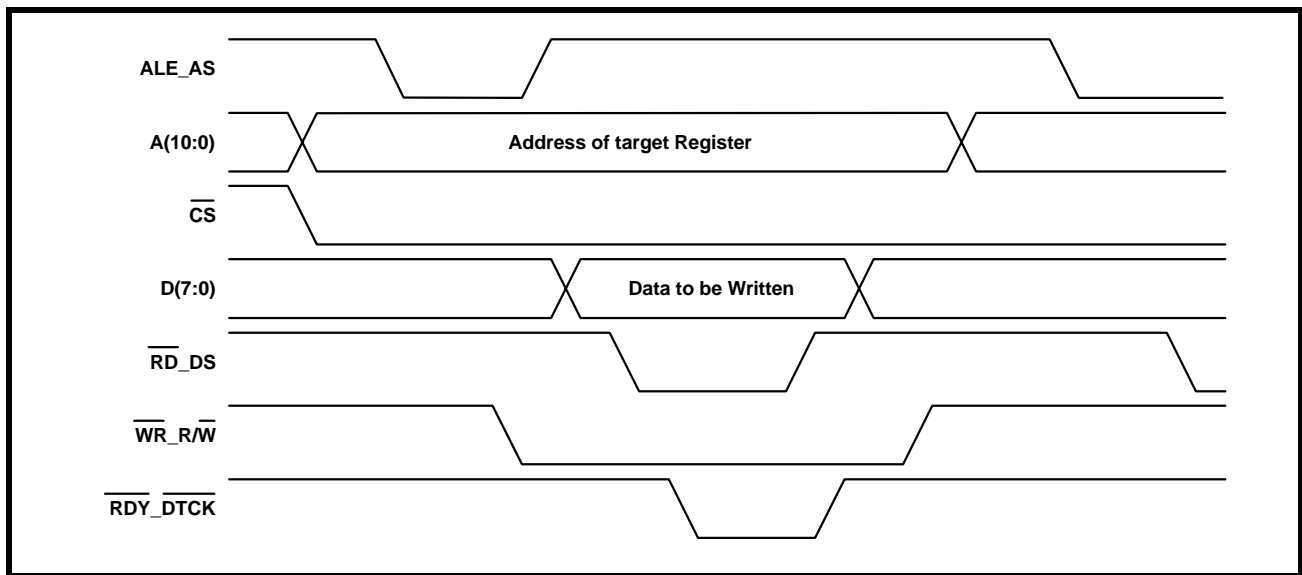
FIGURE 28. ILLUSTRATION OF THE BEHAVIOR OF THE MICROPROCESSOR INTERFACE SIGNAL, DURING A MOTOROLA-TYPE PROGRAMMED I/O WRITE OPERATION
