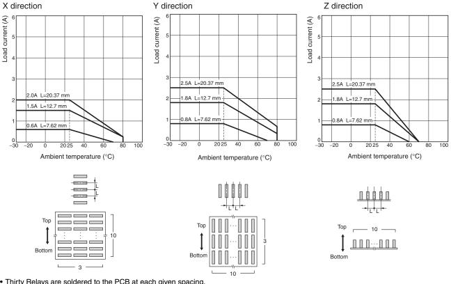
• Thirty Relays are soldered to the PCB at each given spacing.
