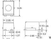
**Note:** A tolerance of ±0.2 mm applies to all dimensions unless otherwise specified.
