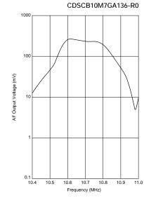
$\begin{array}{l} \text{Input} = 100 \text{dB} \mu \\ \text{fdev.} = \pm 50 \text{kHz} \\ \text{fmod.} = 1 \text{kHz} \\ \text{Vcc} = 5.0 \text{V} \end{array}$
