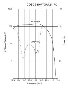
$\begin{array}{l} Input = 100 dB \mu \\ fdev. = \pm 75 kHz \\ fmod. = 1 kHz \end{array}$
