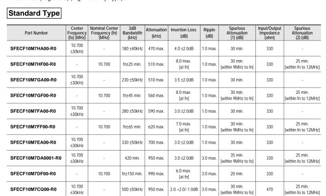
Area of Spurious Attenuation: [within 9MHz to 12MHz]
