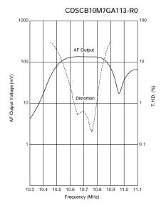
$\begin{array}{l} \text{Input} = 100 \text{dB} \mu \\ \text{fdev.} = \pm 75 \text{kHz} \\ \text{fmod.} = 1 \text{kHz} \\ \text{Vcc} = 1.2 \text{V} \end{array}$
