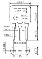
(1) : Input (2) : Ground (3) : Output (in mm)
