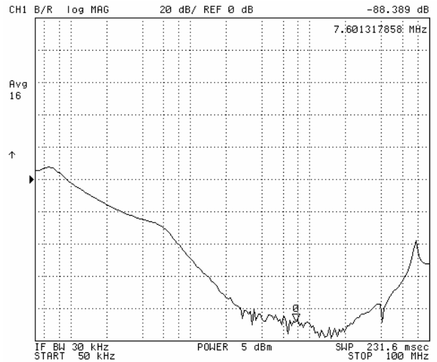
Fig. 3: Common Mode attenuation, 0.05-100 MHz. Source and load resistances are 50 Ω. Two 0.1 μF Y-caps to common line. Vertical scale: 20 dB/div, with zero dB level marked by arrow.
