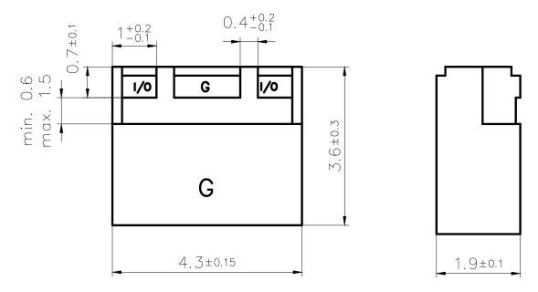
Bottom view onto the solder terminals and side view Marking: EPCOS logo, SC 2326 on top of the filter
