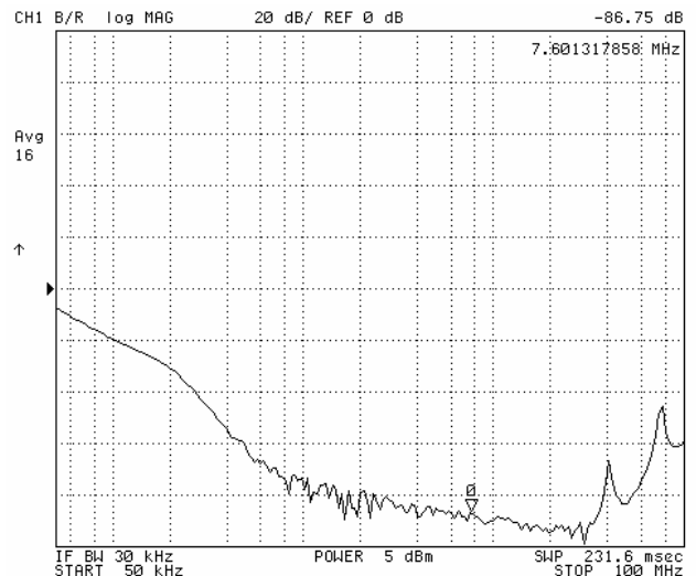
Fig. 4: Common Mode attenuation, 0.05-100 MHz. Source and load resistances are 50 \Omega . Two 0.47 \mu F Y-caps to common line. Vertical scale: 20 dB/div, with zero dB level marked by arrow.
