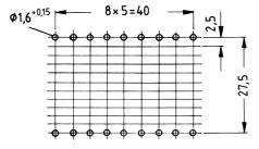
Hole arrangement View in mounting direction
