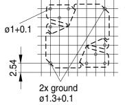
Hole arrangement View in mounting direction
