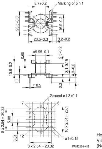
Hole arrangement View in mounting direction (Note half pitch!)
