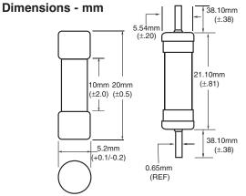
· With TR2 packaging code, lead wire length is 19.05mm
