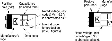
Case sizes W, U, X, V Positive Manufacturer's pole (bar) logo Internal code for production equipment (2 to 3 figures) Date code Rated voltage, (not Capacitance coded)  $V_R = 6.3 V$  (in coded form) is abhreviated as 6
