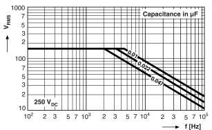
Permissible AC Voltage versus Frequency
