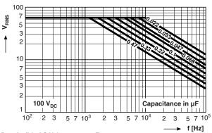
Permissible AC Voltage versus Frequency
