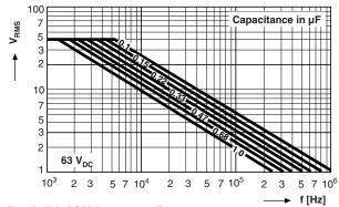
Permissible AC Voltage versus Frequency
