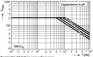
Permissible AC Voltage versus Frequency
