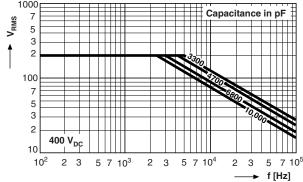
Permissible AC Voltage versus Frequency
