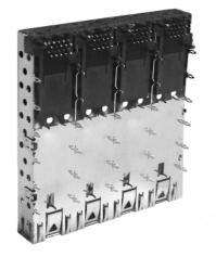
For increased flexibility, Tyco Electronics offers ganged (single Row) SFP cages with integrated connectors that are footprint compatible with its Stacked SFP product line. The connector uses the same press fit technology as incorporated in the stacked SFP cage/connector system, with one-step insertion in the board. Products currently offered are 1x1, 1x4 and 1x6 configurations.
