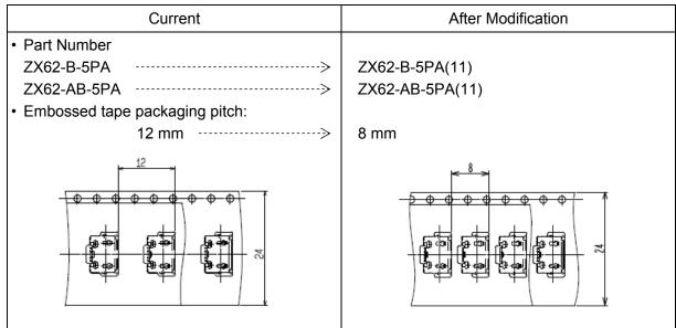
When automatically mounting the changed product, it will be necessary to change the setting of the embossed tape feeding pitch to 8 mm.
