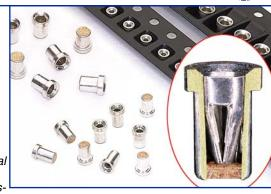
ly been screen printed on pads adjacent to the holes) and the board is reflowed in the same pass as other SMT components. Solder will fill the plated through-holes and achieve solder joints as reliable as wave soldering. The OFP® barrier prevents solder paste from being picked-up inside the contact during pick 'n place assembly. "Overprinting" paste on the solder mask can be used to adjust the volume of paste required to fill each hole.
